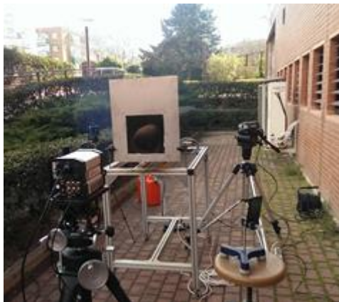
Figure 190 – Determination of thermal properties by means of adapted flash method
