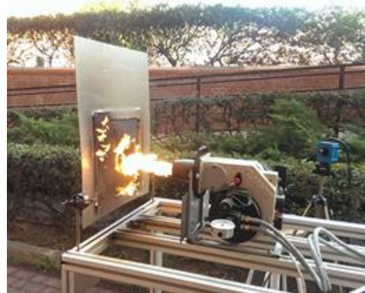
Figure 190 – Determination of thermal properties by means of adapted flash method
