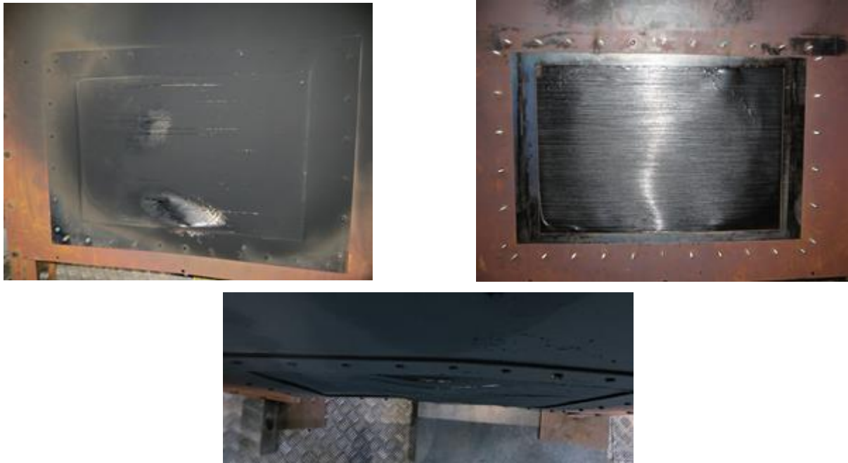
Figure 197 – Panel after standard fire test (Hot face, RHS; Cold Face LHS))
