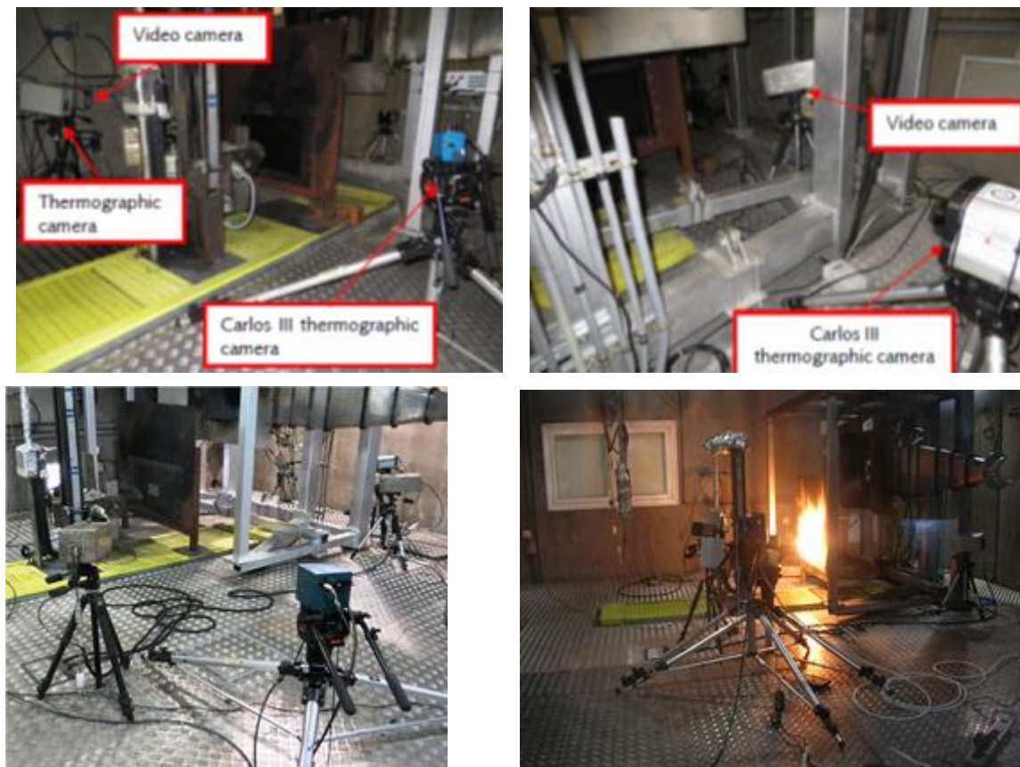
Figure 191 – Fire Test performed with calibrated flame and monitoring equipment
