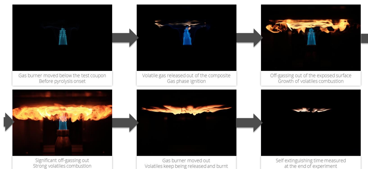
Figure 93 – Overview of the successive events occurring during the fire exposure onto the composite test coupon
