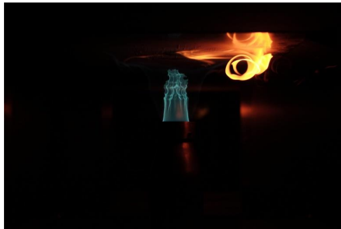
Figure 94 – Internal damage affecting the gas release and ignition on the material surface during test#025
